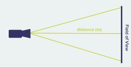
It is important to consider both the mounting height and viewing angle of the camera. If the camera is placed too high, or the horizontal/vertical angle is too big, the recognition accuracy may be reduced.
